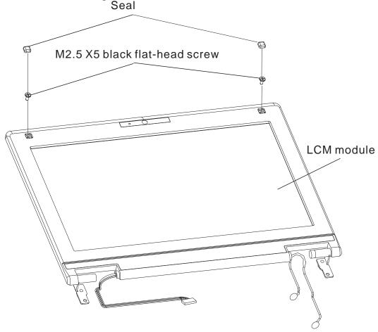
Figure 4-17 Removing the display mask
